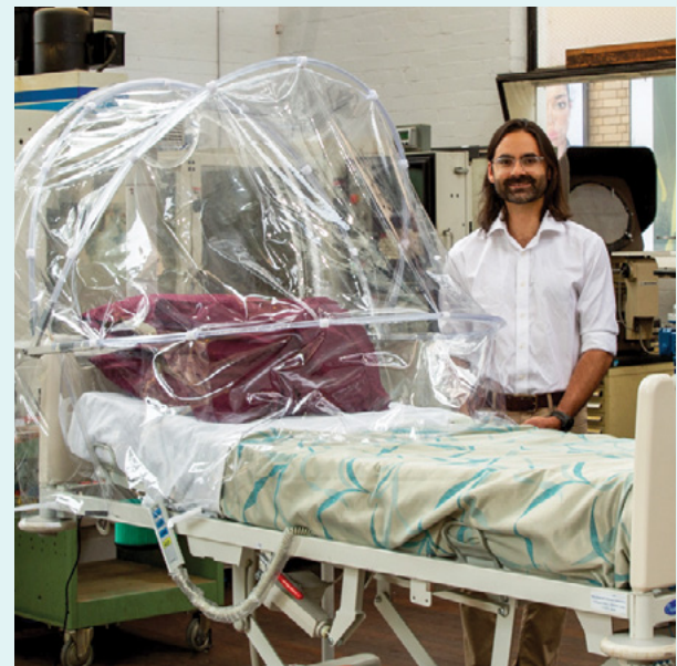
PROFESSOR JASON MONTY AND THE VENTILATION HOOD PROTOTYPE
